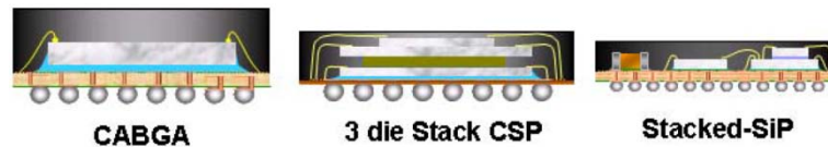
Figure 2.2 Conventional CABGA and thin multi-die stacking or stacked SiP (Lee et al., 2006)
