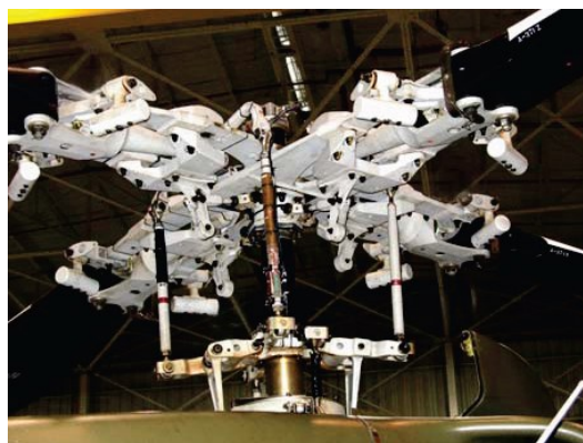
Figure 2.15: Microstrain's energy harvesting, wireless loads tracking pitch link installed on Bell M412 (Arms et al., 2009)
