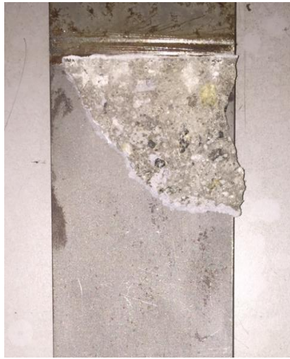
Figure 27: Formation of concrete bulb on steel plate after failure
