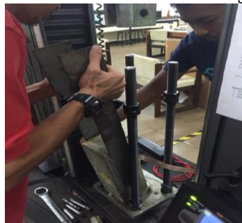
Figure 15: Installation of pull-out test rig
