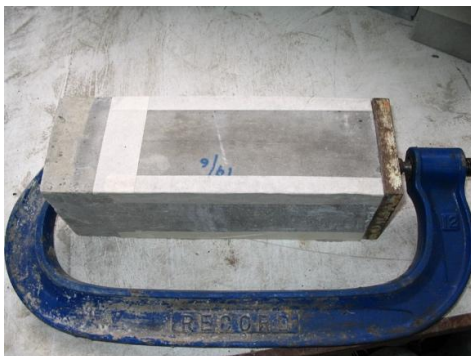
Figure 1: Concrete prisms attached with G-clamp prepared in 2008
