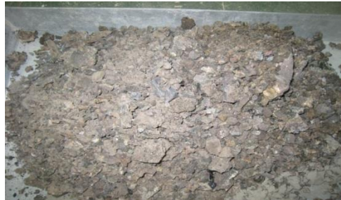
Figure 1: By-product waste - timber clinker aggregate
