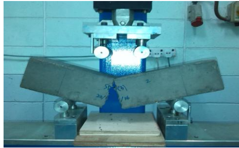
Figure 2: Broken prism sample after flexural test
