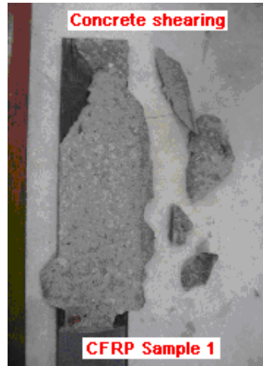
Figure 15: Concrete shearing for CFRP/Con 1
