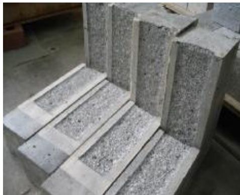
Figure 4: Hacked concrete surfaces
