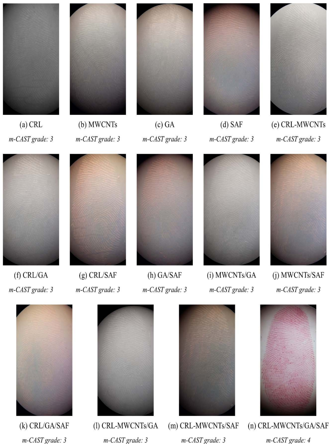
Figure 1. Visualization of latent fingerprints using various combinations of CRL, MWCNTs, GA and SAF observed at 7.5\times magnification (a–n).
