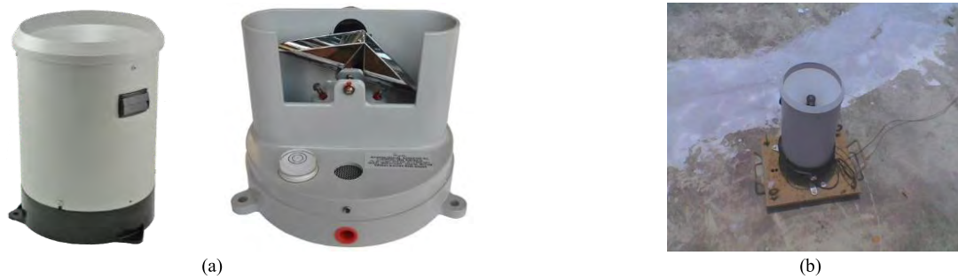
FIGURE 9. Physical photo of rain gauge set with tipping bucket size. (a) Rain gauge set with tipping bucket. (b) Rain gauge after setup.
