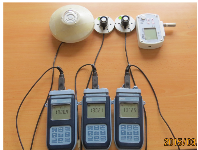
Fig. 4. Assessing the precision of the needed instruments through the calibration test.
