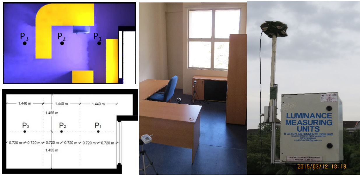
Fig. 3. Position of internal and external illuminance sensors in the furnished test room.
