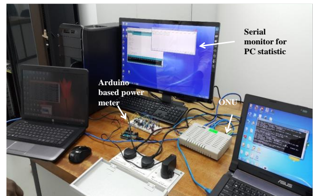
Figure 2 Experimental setup for measuring power consumption of ONU using GPON testbed
