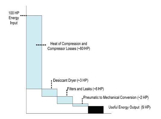
Figure 1.1 Compressed Air Energy Input and Useful Energy Output (Adapted from Northwest Energy Alliance)
