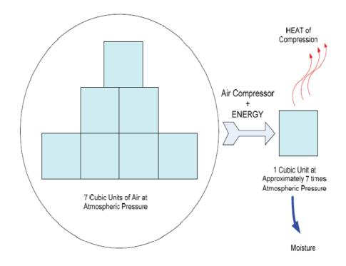
Figure 1.0 Conversion of Atmospheric Air into Compressed Air
