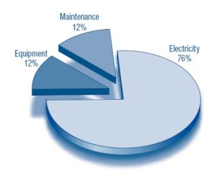
Figure 1.5 Typical Lifetime Ownership Cost of Compressed Air Systems.
