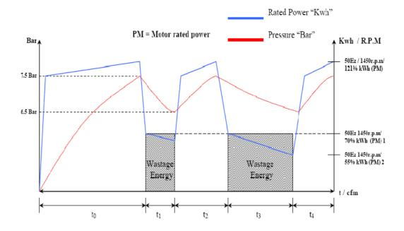
Figure 1.7 Load graph and Air pressure combination
