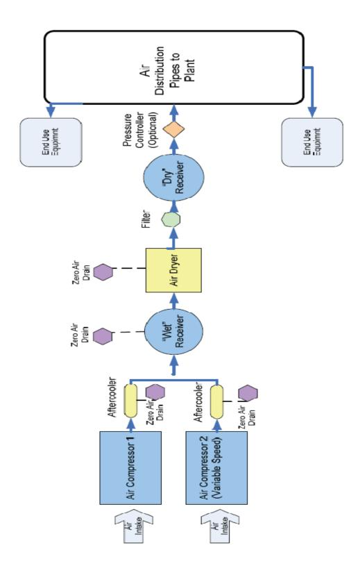
Figure 1.2 Common Air Compressor System Components
