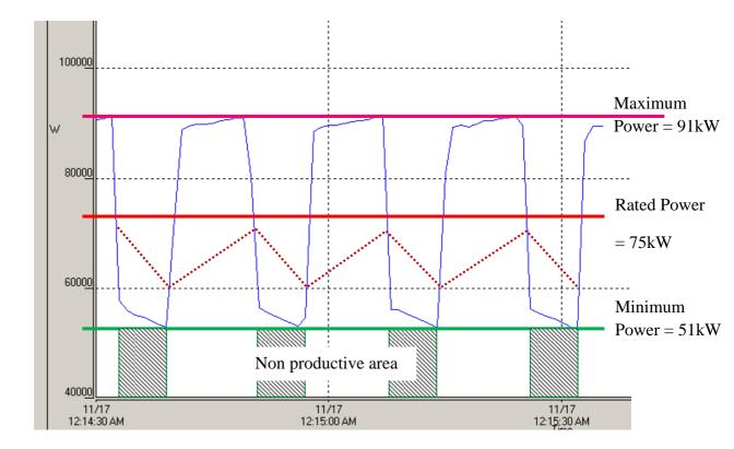
Figure 1.6 Load Graph Cut view on real data
