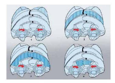
Figure 1.4 Shown Compressed Air process in twin screw compressor
