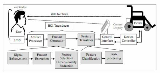
Figure 1.1 A typical EEG-based BCI components [16].
