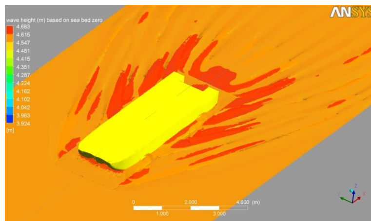
Fig. 6: Wave height contour around ship hull
