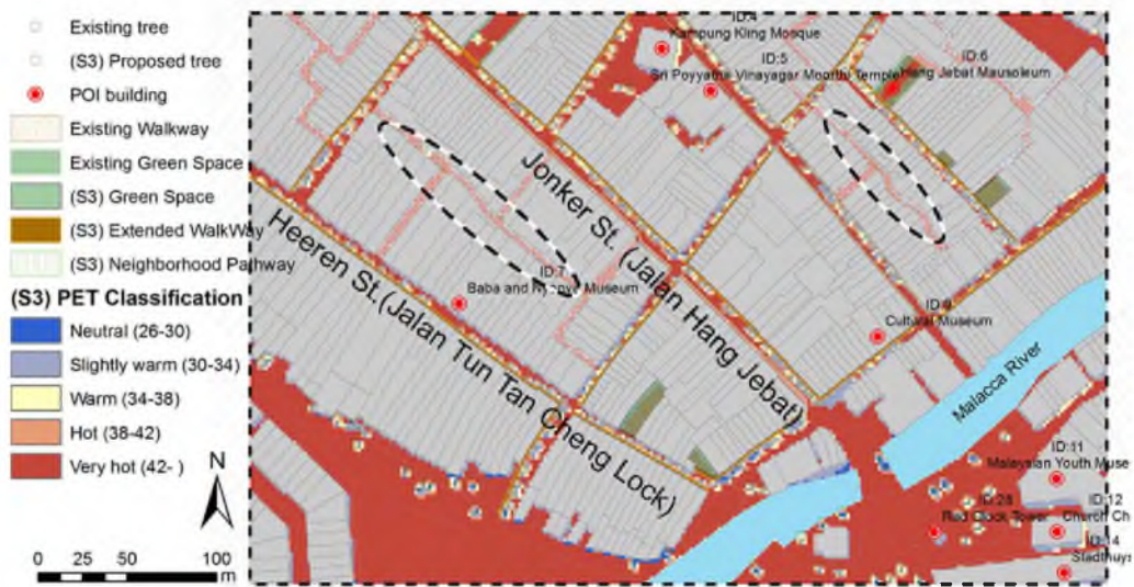
(b) PET classification at 2 pm and at 1.5 m above the ground level (case 3).
