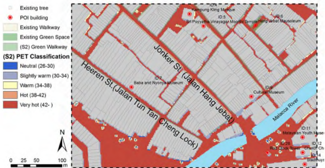
(a) PET classification at 2 pm and at 1.5 m above the ground level (case 2).
