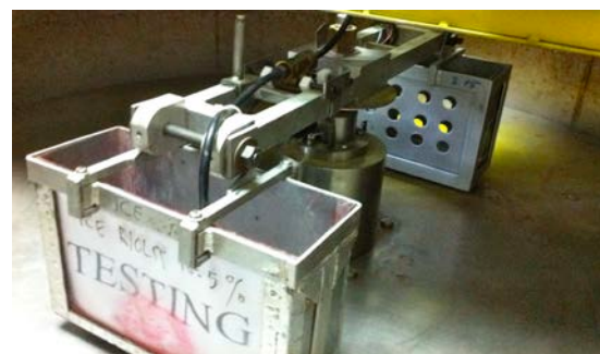
Fig.2 Section view and inside view of UKM mini centrifuge apparatus
