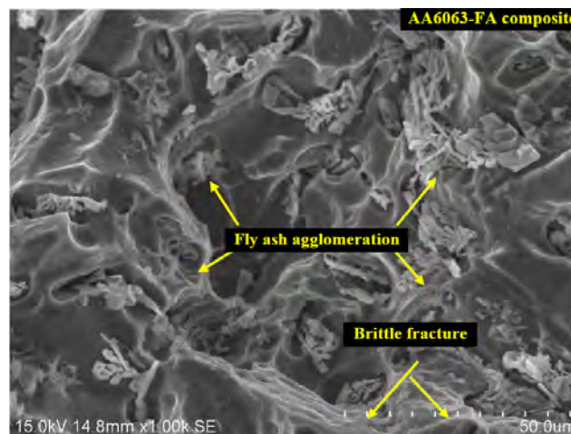
Figure 13. VP-SEM fractography of AA6063-FA composite with 12 wt % fly ash.
