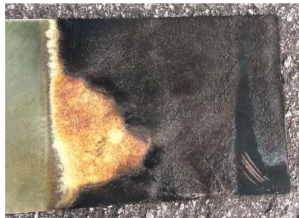
Figure 4 Delamination of fibres
