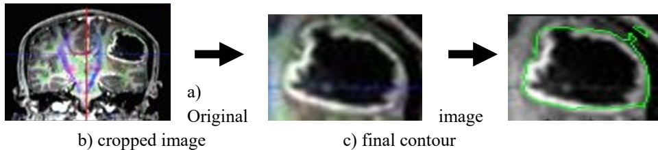
Figure 3.2: The process of edge detection on the brain tumor for front view image
