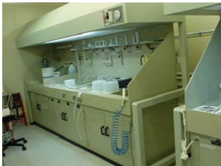
Figure 3-3: Etching baths at IMB-CNM clean room
