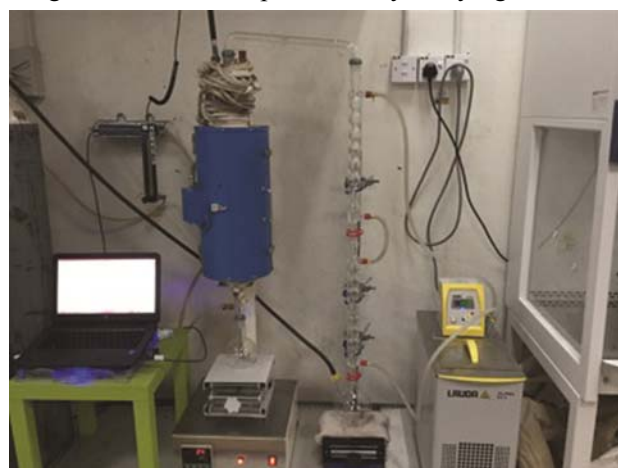
Fig. 1 — Pyrolysis diagram for setup of a slow pyrolysis process. [(1) Electric furnace and Quartz glass reactor; (2) Temperature controller; (3) Thermocouple, connected to data logger system; (4) Nitrogen gas; (5) Glass tube connector; (6) Condenser; (7) Receiving flask; (8) Water cooling circulator; and (9) Safety liquid collector]
