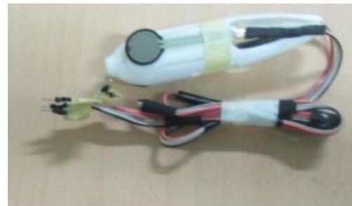
Figure 3 TREMORX with FSR (SN-FRC-0.5) and Flex sensor (SN-FLX-FC)
