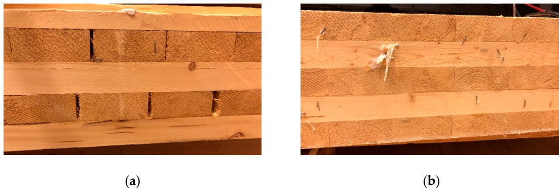
Figure 14. (a) Air gaps in the laminate layers of CLT. (b) No edge-bonding of CLT.
