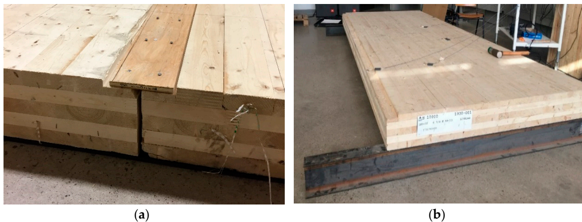
Figure 1. (a) Two CLT panels connected by a thin wooden lath. (b) One CLT panel simply supported on two I-steel beams.
