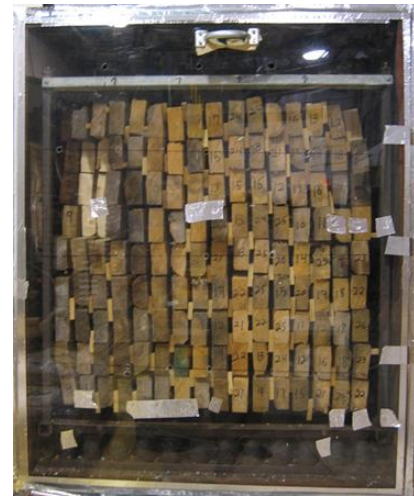
Figure 4: Vertical placement of wood in the treatment chamber
