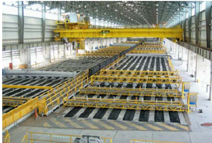
Figure 1 : A horizontal anode baking furnace in operation [2]
