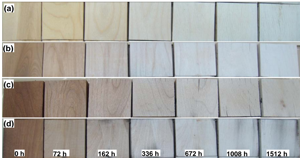
Fig.1 Visual appearance of tangential surfaces of birch, untreated and heat-treated at different temperatures during weathering: (a) untreated, (b) heat-treated at 195°C, (c) heat-treated at 205°C, (d) heat-treated at 215°C
