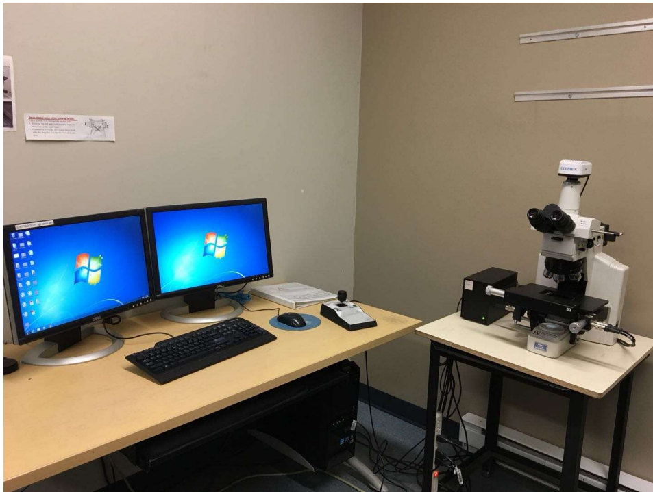
Figure 3.2: Clemex image analysis system with Nikon Eclipse ME600 optical microscope.
