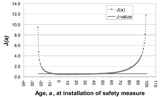
Fig. 2. Individual J -value, J ( a ), against age, a , at the time of installation of the safety measure: worked example of Appendix D. (The true J -value is marked on as a horizontal line.)
