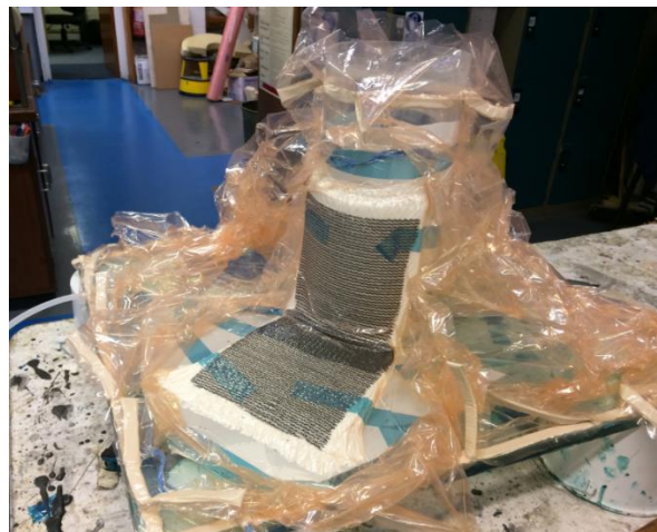
Fig. 4.13: The vacuum infusion process of the experiments
