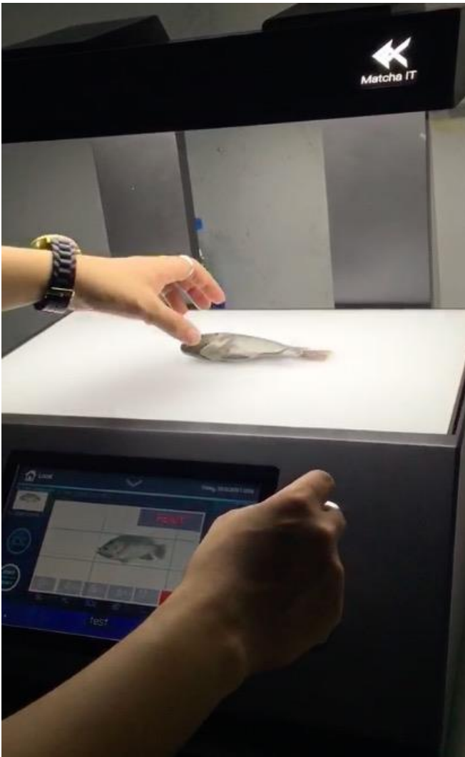
Figure 2.4 The automatic recording system (Matcha IT, Thailand) was used to monitor individual tilapia growth
