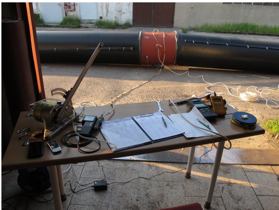
Figure 8 Measuring station with micromanometers and Pitot tube
