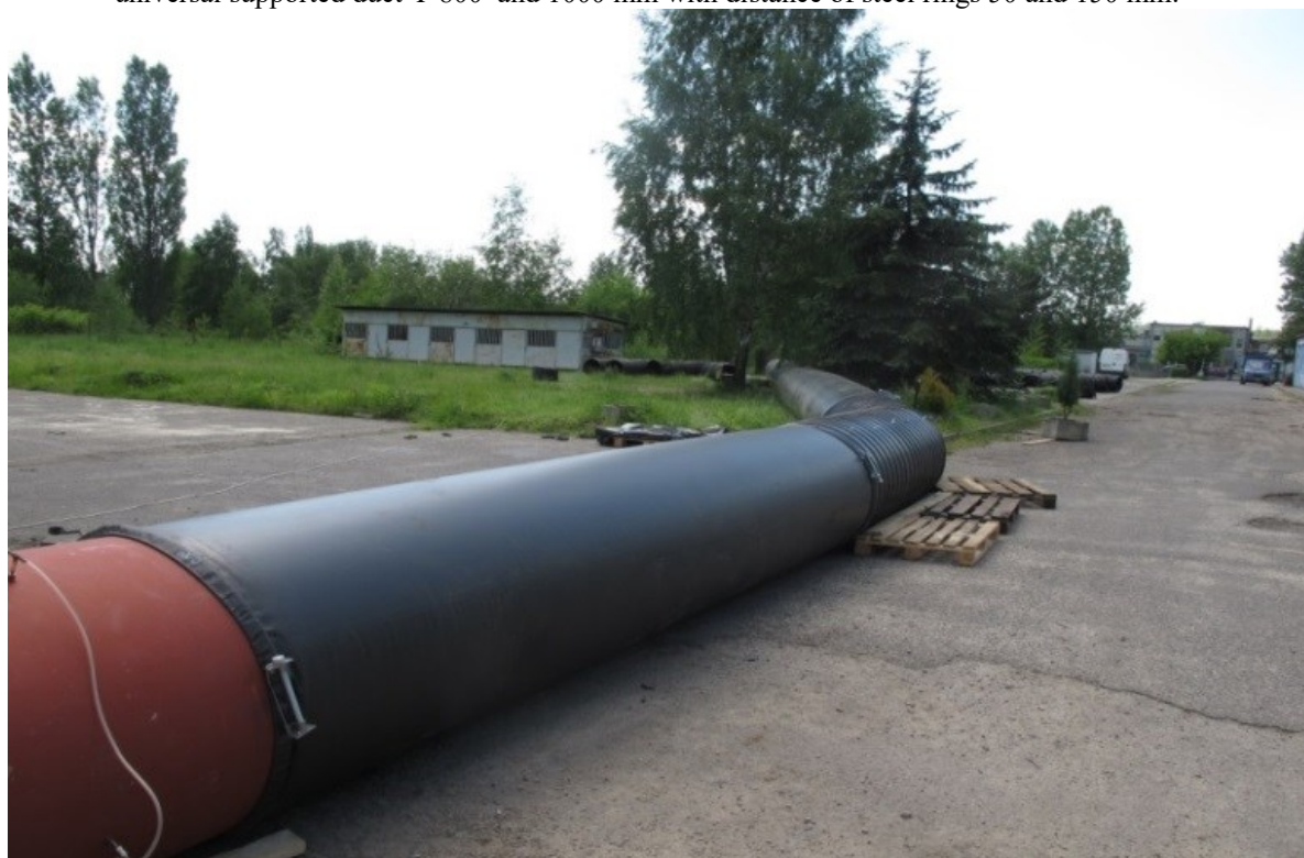
Figure 6 Overpressure unsupported duct with 30° bend
