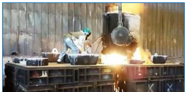
Fig. 8. There are almost no emissions, exhalations during pouring
