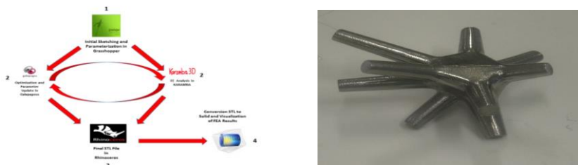
Fig. 5: From left to right. (a) Overview of Optimization Process, (b) Final Metal 3d-Printed Node by using Fatness Parameter Method.
