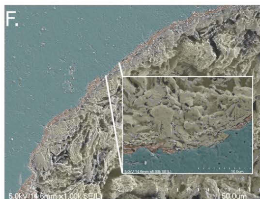
Figure 3.5 SEM images of a cross section of cured coated microspheres (A) Batch 16, mean coating thickness = 19 \pm 0.8 \mu\text{m} (B) Batch 17, mean coating thickness = 16 \pm 2 \mu\text{m} (C) Batch 1, mean coating thickness = 9.6 \pm 2 \mu\text{m} (D) Batch 2, mean coating thickness = 10 \pm 1 \mu\text{m} . (E) Batch 12, mean coating thickness = 6.3 \pm 2 \mu\text{m} and (F) Batch 13, mean coating thickness = 4.2 \pm 0.3 \mu\text{m} . False color was added to highlight the different regions in the images, color scheme is as follows: Blue: epoxy, orange: coating, yellow: MSC microspheres core.
