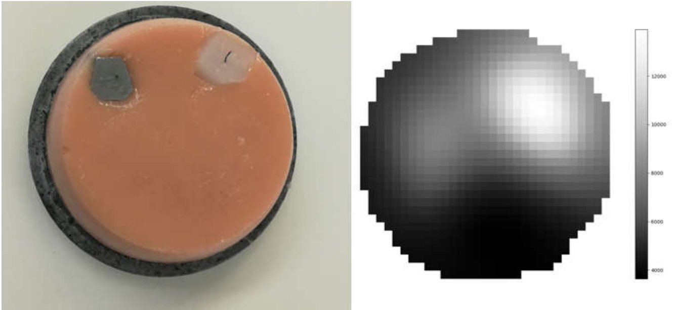
Figure 4.8: Left: location of the inclusions within the phantom. Inclusion 1 is the stiffer of the two. Right: the corresponding slice of the DICE reconstruction showing the location and relative stiffness of the two inclusions.
