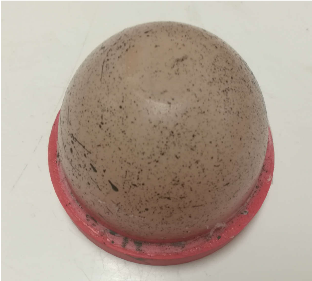
Figure 3.2: The tissue-mimicking silicon breast phantom used for this study, with the random speckle pattern for DIC applied.
