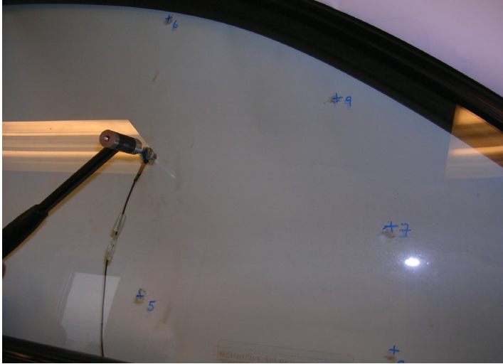
Figure 4.1 Driving point mobility test on side glass of passenger car
