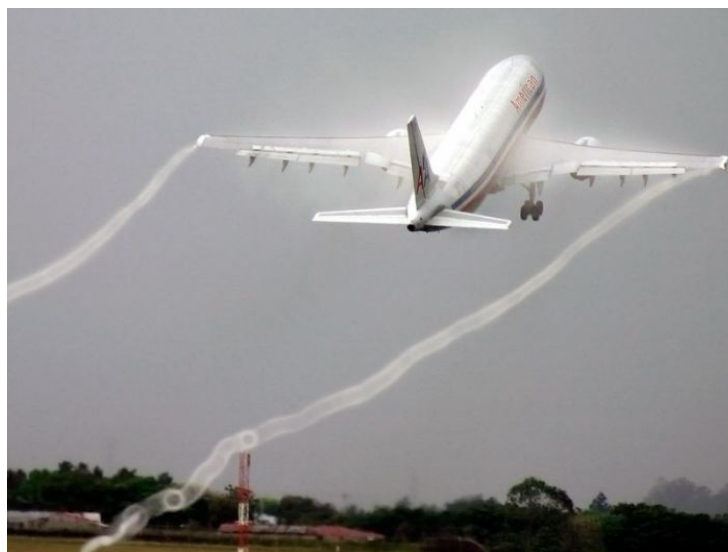
Figure 1.1 Wing tip vortices at take-off [115]
