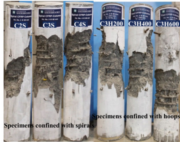
Figure 2-5- Overview of the CFRP RC column specimens after failure (Afifi et al.,2014)
