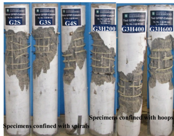
Figure 2-4- Overview of the GFRP RC column specimens after failure (Afifi et al., 2014)
