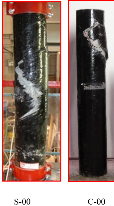
Figure 3-4 – Failure modes of the concentrically loaded columns (S-00, C-00)
