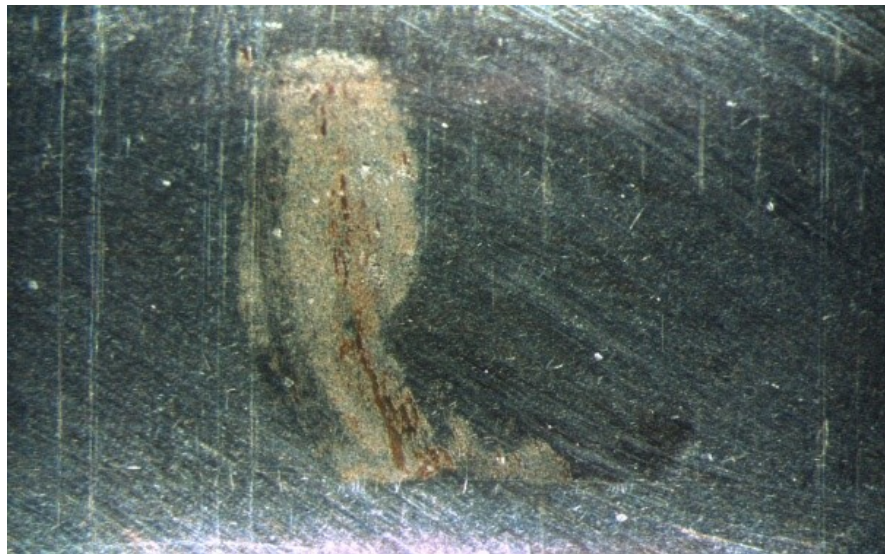
Figure 5: Micrograph showing the deterioration of a steel cylinder at the contact point after 2250 cycles of insertions without lubrication (run 1).
