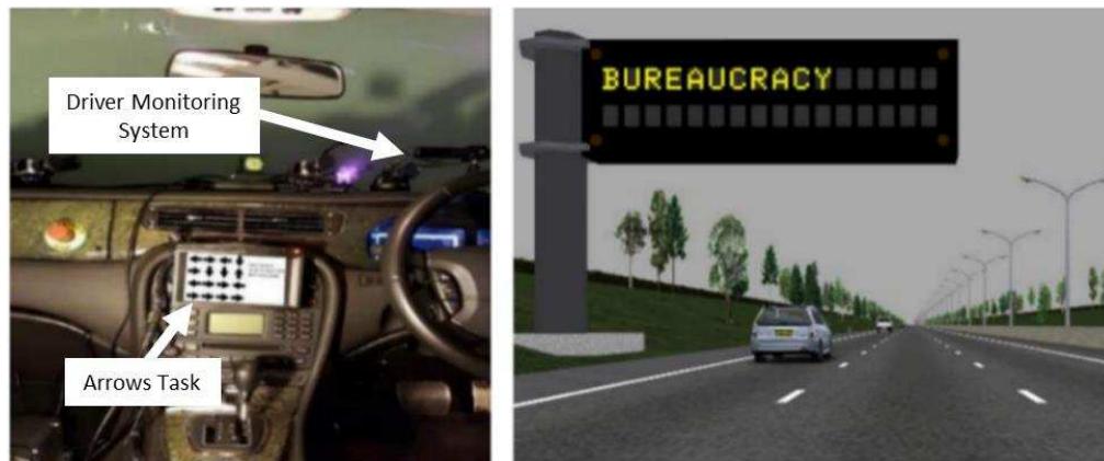
Figure 1 - Example of the Arrows NDRT (left), the position of the task in the vehicle (middle) and the VMS (right).
