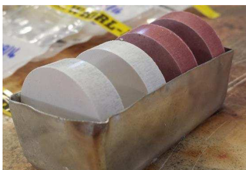
Figure 4: Image of the four 28x7 disks of A-CSA #1-4 before being fired in a platinum crucible, with A-CSA #1 located at the bottom left of the image, followed by A-CSA #2, #3, and #4 towards top right. A-CSA #3 and #4 are red due to the presence of iron.
