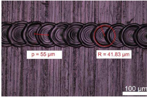
Figure 9: Optical micrograph of the top surface of a single track. Process parameters: Q = 190 W, t_e = 150 \mu s, and p = 55 \mu m. Predicted melt pool radius ( R_m ) from Rosenthal solution is 38 \mu m and from 1D model is 290 \mu m, compared with 42 \mu m measured experimentally.
