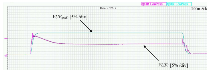
Figure 10. Operation under two-phase voltage drop ( V_{ga} = 0.73 p.u. and V_{gc} = 0.65 p.u.): Voltage unbalance factors.
