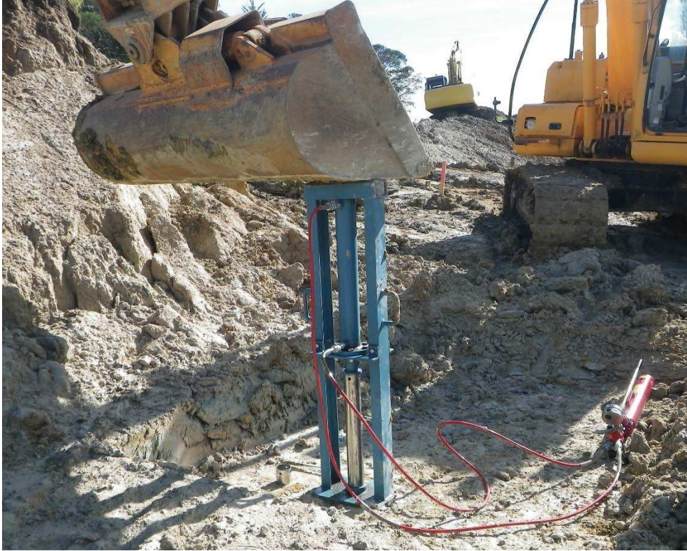
Figure 5: Rig and jacking frame used for Shelby tube same collection.
