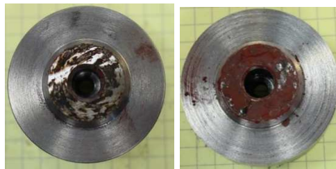
Figure 17: Example of the exposed metal seen post-test.
