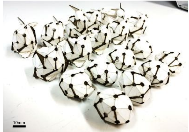
Fig. 21. Self-folded bunny and egg shapes. The scale bar is 10 mm.
