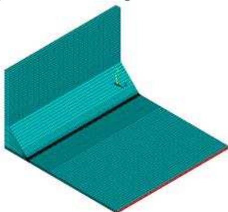
Figure 5. Examples of linear elastic FE models (a) and (b) solved using a 2-dimensional models (c) solved using a 3-dimensional models following the standard solid-solid sub-modelling procedure.
