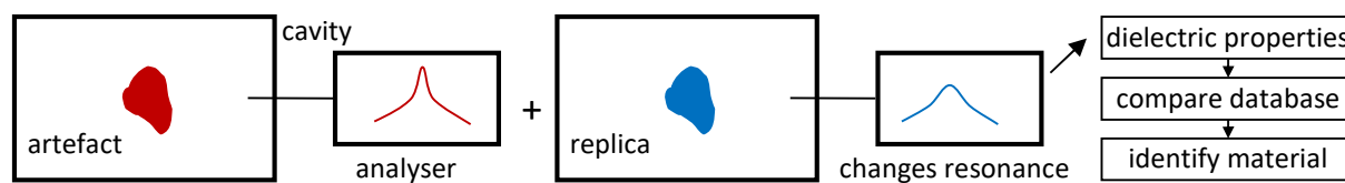
Figure 1. Principle of Dielectric Replica Measurement (DRM)
