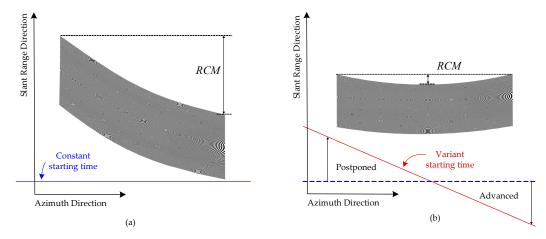
**Figure 7.** Effect of a variable starting time for the receive window. (**a**) The echo acquired by the squint mode with a constant starting time for the receive window represented by the blue line. (**b**) The echo acquired using the same mode but with a starting time that varies according to the red line, where the starting time is postponed during the first half of data recording and is advanced during the latter half.
