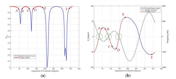
**Figure 14.** The spatial variance index and ground squint angle curves when observing Wenchuan in full orbit. (a) The spatial variance index  $g_{var}$ ; (b) the ground squint angle  $\theta_g$ . The black dashed line is the Doppler centroid frequency, which has three intersection points with the ground squint angle curve at  $\theta_g = 0$ . These three points are highlighted by green circles, corresponding to the broadside mode in Figure 13a.
