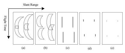
**Figure 9.** Conceptual basis for the proposed squint mode GEO SAR imaging algorithm. The echo signals after bulk range walk correction are demonstrated as subfigure (**a**). Then first-order filtering is applied, and the results are presented as (**b**). RCMC and other range operations together make the signals into (**c**). Partial dechirp and relevant operations shorten the azimuth span, which is shown in (**d**). Lastly, azimuth compensation produces the final images (**e**).
