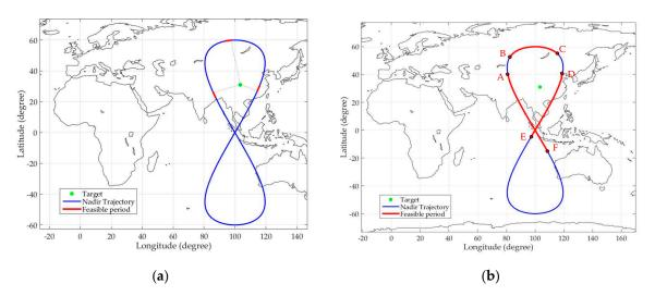
the nadir trajectory, the red lines represent the feasible observation durations corresponding to the respective observation modes, and the green point represents the target location.
