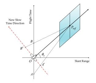
**Figure 8.** Equivalence between the broadside mode and the squint mode for a reference target  $P_{ref}$  using a variable starting time for the receive window.
