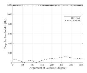
**Figure 6.** Doppler bandwidths of GEO SAR and low earth orbit (LEO) SAR with an azimuth resolution of 5 m based on Equations (7) and (10). We consider L-band GEO SAR in orbit with an inclination angle of 60°. The parameters employed for LEO SAR are the same as those of L-band ALOS-2 [19]. In this case, the Doppler bandwidth of GEO SAR is nearly 1/10 that of LEO SAR.
