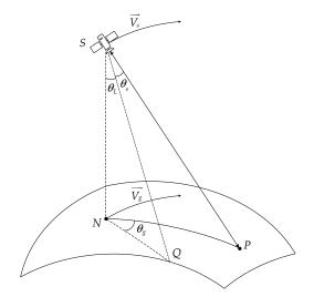
**Figure 12.** The observation angle relationships in GEO SAR. *S* denotes the satellite position, *P* is the target position on the ground, and *N* is the nadir point. *SP* is the beam-center line. *SNQ* is the zero-Doppler plane, *SNP* is the squint plane,  $\theta_L$  is the elevation angle,  $\theta_s$  is the squint angle, and  $\theta_g$  is the ground squint angle.
