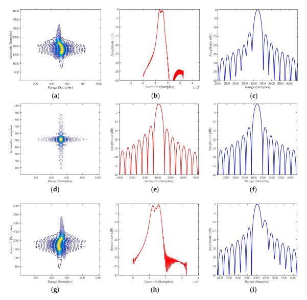
**Figure 16.** Imaging results of the 2D nonlinear chirp scaling (CS) algorithm [18]. The first (**a**–**c**), second (**d**–**f**), and third (**g**–**i**) row correspond respectively to points  $T_1$ ,  $T_2$ , and  $T_3$  illustrated in Figure 15. The first (**a**,**d**,**g**), second (**b**,**e**,**h**), and third (**c**,**f**,**i**) column represent contour maps, azimuth profiles, and range profiles, respectively.
