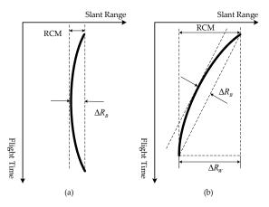
Figure 3. Range cell migration (RCM) of GEO SAR: (a) Broadside looking mode; (b) squint looking mode.
