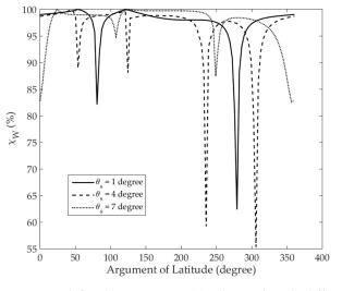
**Figure 4.** Values of ratio  $\chi_W$ , defined in Equation (5), obtained with different squint angles  $\theta_s$ , which include 1, 4, and 7 degrees. Because of the high orbital height, the maximum value of  $\theta_s$  is approximately 7° for GEO SAR.
