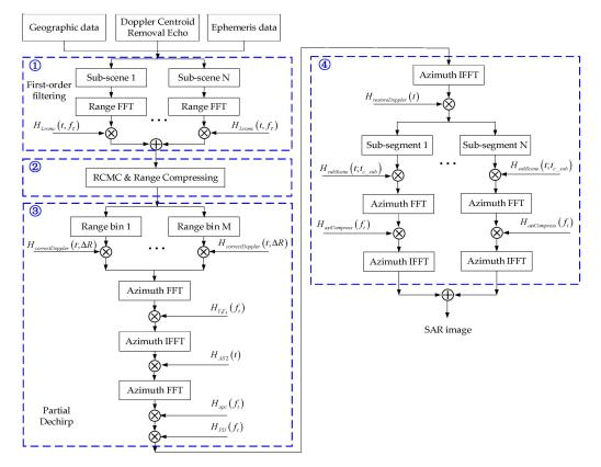
**Figure 10.** Flowchart for the proposed squint mode GEO SAR imaging algorithm, which is composed of four steps. Step 1 is first-order filtering. Step 2 includes range cell migration correction (RCMC) and range compression. Step 3 implements partial dechirp. Azimuth compensation is accomplished in Step 4.
