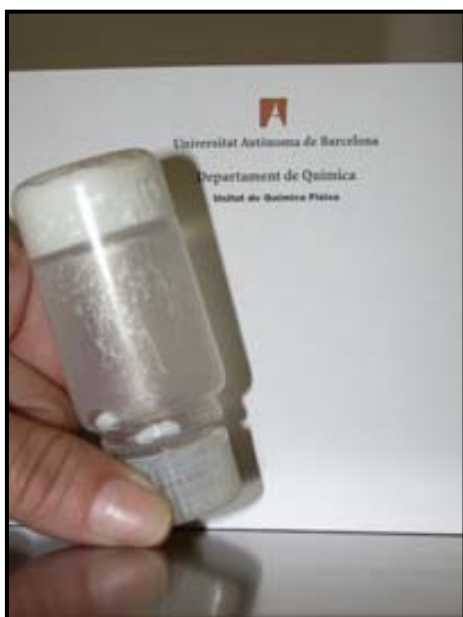
Figure 4.4.3. Final quasi-solid \text{TiO}_2 paste with “cheese-like” appearance (from [\text{Cho}]_2\text{TiF}_6 medium) in the 30 ml Teflon-covered plastic reactor employed. Titania yield was almost 100%; \text{TiO}_2 mass obtained/volume of reaction mixture was 1g / 10ml, approx.
