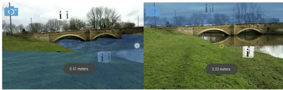
Fig. 11. Flood level is displayed between the set min/max values. Sliding the flood plane vertically interpolates between the two extremes.
