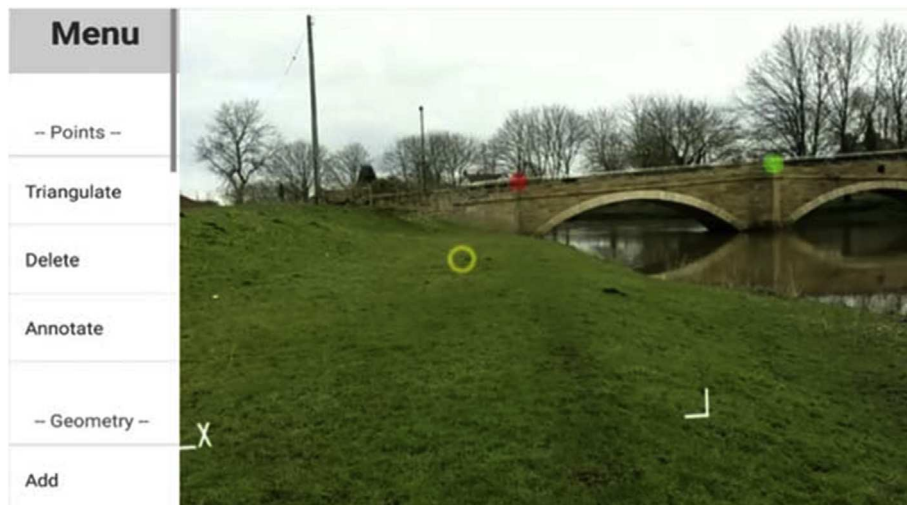
Fig. 4. Browser/Authoring tool. AR tracking showing side menu, interaction annulus, and two triangulated points.
